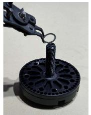
2. Remove hinge pins with pinch pin. \*\* one side of the center hinge pin is press fit in to the center block. Make sure this pin is driven out the right way by tapping the center hinge pin out of its location. if you then see a press mark on the cylindrical part of the pin then you can drive the pin fully to that side. If you don't see this mark, then drive out the pin the opposite side\*\*
