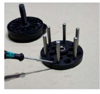
2. Inspect main bolt thread and helicoil in base plate for wear.
