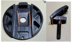
4. Apply a small amount of anti sieze ceramic paste to all hinge surfaces and reassemble the mount.
